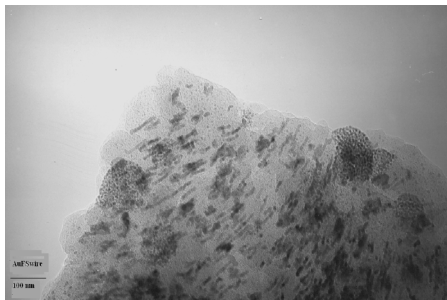
Figure 1. TEM image of Au-nanowires obtained following exposure of \text{HAuCl}_4 encapsulated in FSM-16, and synthesized by CVD method, to \gamma -rays at 300 K.
